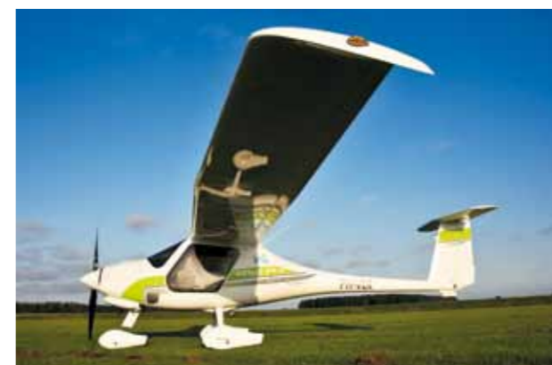
ABOVE: the heavier, faster Virus is distinguished from the microlight Alpha by its downturned wingtips and extended spats
