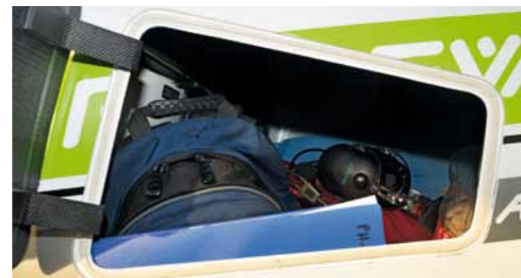
LEFT: reached from outside, the small baggage bay will take a maximum of 25kg
