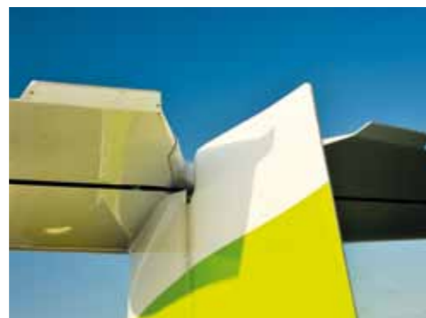
ABOVE: constant-speed MT propeller helps bestow impressive short-field and high-speed cruise performance BELOW LEFT: along with carefully profiled spats, the composite undercarriage bow generates minimal drag BELOW RIGHT: an unusual Pipistrel detail – moulded-in fixed tabs, designed to trim out elevator forces
